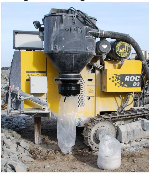
ILMEG Bag Handling Solution. Designed for improved productivity, improved working conditions and cleaner environment in the construction and mining industry.
