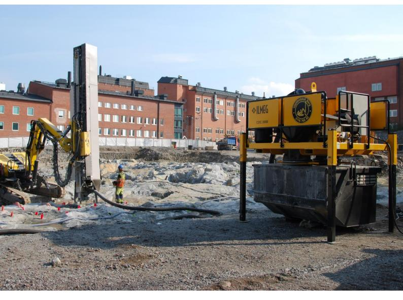
Heavy duty electrically powered dust collector system, designed for extreme demand on dust control and improved working conditions in the construction and mining industry.
