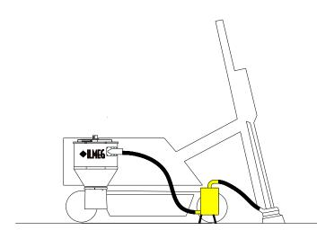
In-line use of the SCS 3000. Used together with a standard dust collector.
